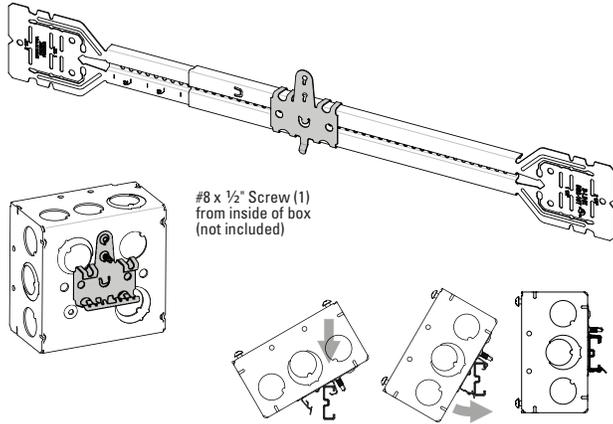
When BB2-16T or BB2-24T is used on metal studs in Canada, at least one (1) listed Box Stabilizer must be installed on the electrical box closest to the center of the bracket to maintain cUL listing.
