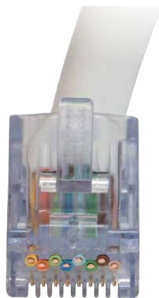
Front of connector after termination and wires are trimmed flush.
