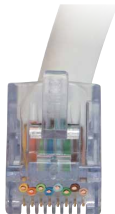
Front of connector after termination and wires are trimmed flush.
