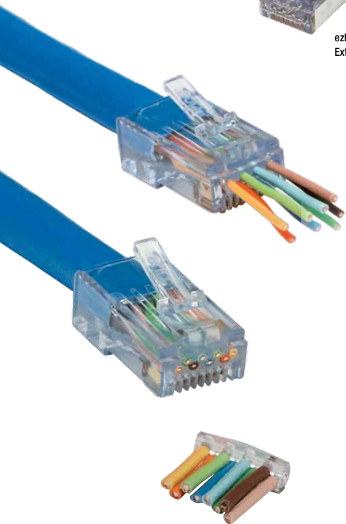
Wires protrude from the front of the connector before being trimmed flush.
