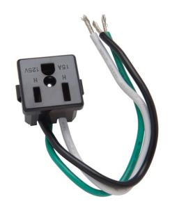
Snap-in receptacle, three wire grounding outlet with 6" leads,No. 14 AWG, 105° plastic. 15 amp, 125 volt, Black.
