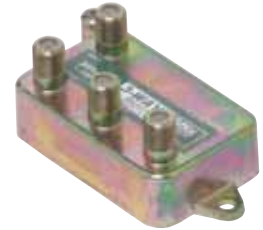
201-261 3-Way 1GHz 90dB Vertical RF Balanced Splitter
