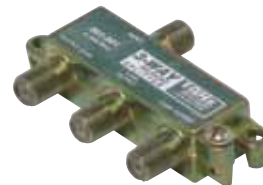
201-201 3-Way 1GHz 90dB RF Balanced Splitter
