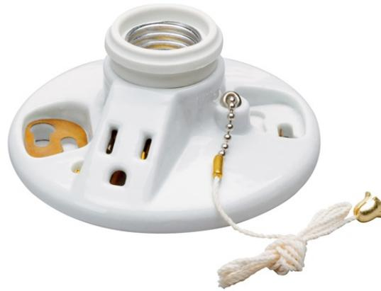
Medium base, porcelain, pullchain, 2 terminals with tri-drive screws, 15 amp, 125 volt, grounding receptacle, fits 3 1/4" and 4" boxes with cage neck. White.
