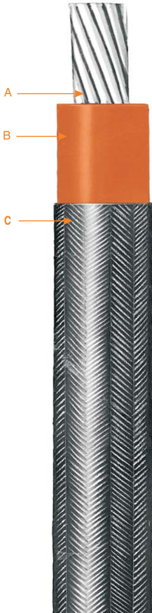
A Uncoated, Stranded Copper Conductor B Insulation—Okonite #16 and #14 AWG 2/64"; #12 AWG through #9 AWG 3/64" C Finish—Nylon Braid with Lacquer Overall
