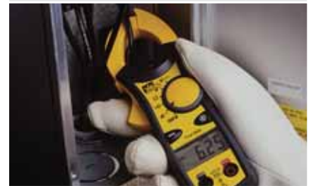
Compact jaw for use in tight locations
