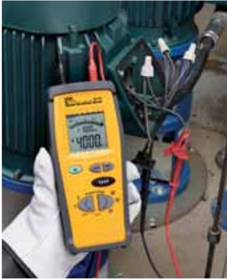
Tests insulation on motor windings
