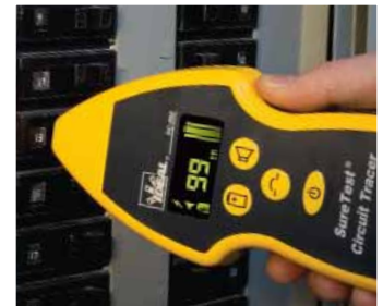
In Breaker Mode, receiver identifies the correct circuit to which the transmitter is connected.
