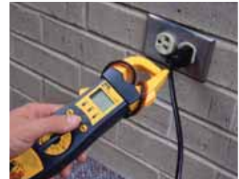
2: Non-Contact Voltage Tester Use it for one-touch indication of power without test leads.
