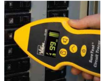
In Breaker Mode, receiver identifies the correct circuit to which the transmitter is connected.
