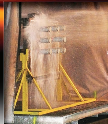
Hose stream test
