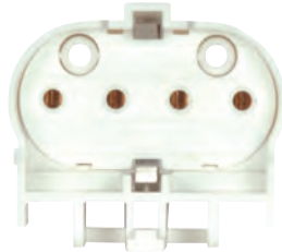
80-1601 Shunted Horizontal Snap-In Mounting for Electronic Ballasts Bottom Push-In Wiring 1 5/8" H x 1 7/8" W x 7/8" Dia. 660W-600V
