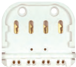
80-1605 4-Pin Long Twin Tube Lampholder Molded White Thermosetting Urea Copper Alloy, Double-Edge Contacts Push-In Wiring Accepts 18 AWG Leads - Solid, Solder Dipped or Twisted, Tinned & Fused 1 7/8" H x 2 1/8" W x 7/8" Dia. 660W-600V
