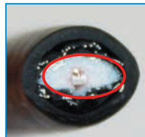
Bad Oval dielectric
