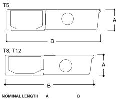
1 1/16" (27mm) 5" (127mm) **T5** Т8 1 1/4" (32mm) 4 1/2" (114mm) T12 1 3/4" (32mm) 5 1/8" (131mm)
