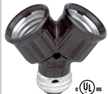
90-1121 Brown 90-2465 Ivory Single to Twin Lampholder Overall Height 2 3/4" - Ext. 2" 660W Max. Total-250V
