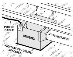
Plan to supply the unit with proper line voltage and appropriate power cable.
