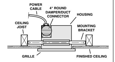
This unit can be installed anywhere between joists using mounting brackets provided.
