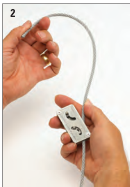
2 Loop wire rope through/around support
