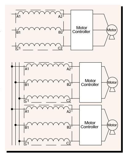
reduction properties coupled with the reactors ability to smooth out voltage transients helps to reduce the instances of motor control faults, which will increase the operating time and effectiveness of your equipment.
