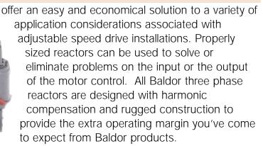
The reactor acts as a current limiting device and performs a similar function to the familiar DC Choke. The reactor will act as a filter to the power waveform to attenuate electrical noise
