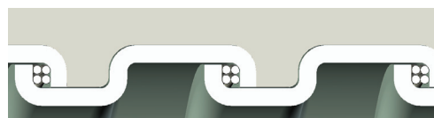
Square-Locked Design with cord packing 5/16" through 1-1/4"
