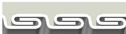
Interlocked Design 1/4" and 1-1/2" through 4"
