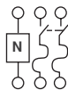
Fig. A MHF221N, MHF222N, MHF223N, MHF224N, MHF221NR, MHF222NR, MHF223NR, MHF224NR 2 pole, 3 wire
