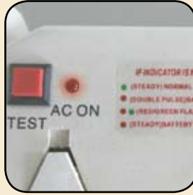
Steady Red = Battery disconnected Double-Pulse Red = Battery failure
